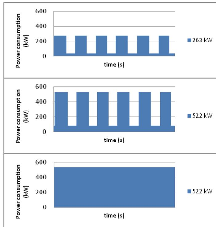
Figure 3: Load/unload profiles
