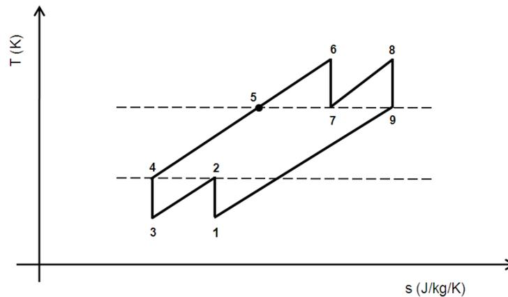
Figure 4: Ideal gas-turbine cycle
