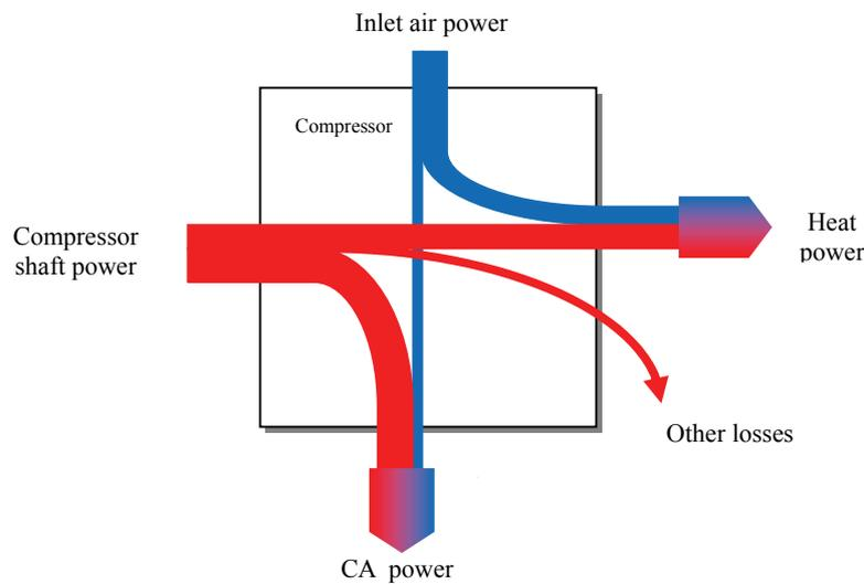
Figure 1: Energy balance of compressor
